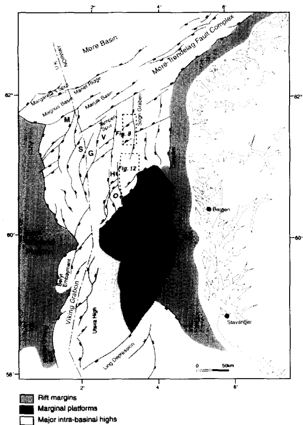
Fig. 2. Major structural elements associated with Jurassic extension in the northern North Sea. The location of fault-blocks referred to is as indicated. G, Gullfaks Fault-block; H, Huldra Fault-block; M, Magnus Fault-block; O, Oseberg Fault-block; S, Statfjord Fault-block; V, Visund Fault-block.
